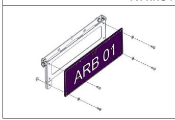
9. Using 4 X SStl M6 button head screws, 4 x M6 washers SStl and M6 flange nuts attach the number plate to the pivot bracket.
