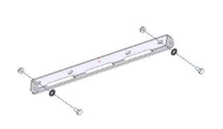
1. Fit the base bracket to the bull bar using 2 X M6 x 20 bolts, 2 X M6 flat washers and M6 flange nuts. Centralise the bracket, ensure it is level to the bar and tighten to the specified torque.
